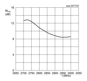
$V_{DS}$  = 32 V;  $P_L$  = 200 W;  $I_{Dq}$  = 100 mA;  $t_p$  = 300  $\mu$ s;  $\delta$  = 10 %.
