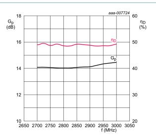
$V_{DS}$  = 32 V;  $P_L$  = 200 W;  $I_{Dq}$  = 100 mA;  $t_p$  = 300  $\mu s;$   $\delta$  = 10 %.
