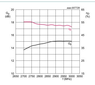
$V_{DS}$  = 32 V;  $P_L$  = 220 W;  $I_{Dq}$  = 50 mA;  $t_p$  = 3000  $\mu s$ ;  $\delta$  = 20 %.
