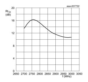
$V_{DS}$  = 32 V;  $P_L$  = 220 W;  $I_{Dq}$  = 50 mA;  $t_p$  = 3000  $\mu s; \, \delta$  = 20 %.
